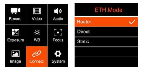
2. Connect the camera to a router with an Ethernet cable, then connect the router to the computer with Ethernet cable or Wi-Fi. (Note: Camera and PC should connect to the LAN port of router, not WAN port)
