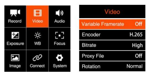
• Variable Frame Rate (VFR): With VFR you can set a different frame rate for capturing based on the Project FPS for recording, in this way you can get a slow-motion or fast-motion footage.
