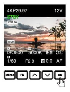
• **AEL (F1)**: Press **F1** to lock the exposure, then press again to unlock
