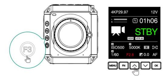
• EV: Press DOWN to set EV, then press Up / Down to adjust the value, and OK to confirm.
