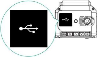
4. PC will detect the camera and shows it as external storage device. You can access & manage the files in the CFast card inside the camera.
