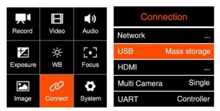
3. Connect the camera to a computer with an USB Type C cable, an "USB" icon would show up on LCD screen, then it's connected successfully.
