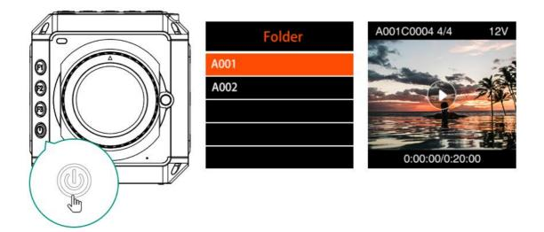
Press **OK** button to play the selected footage. When the footage is being played, press the **Up** / **Down** button to speed up / slow down (2x faster / slower).
