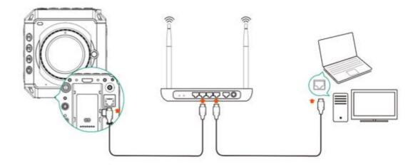
3. Check the **Connect** – **Network** setting, and there will show the IP address of the camera on **ETH.IP** item (e.g. 192.168.1.101) if the connection is OK.
