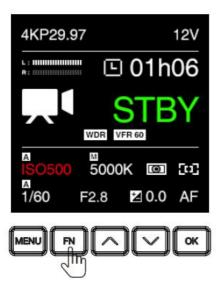
• Shutter: Press UP to set shutter speed / angle (refer to 2.5 Exposure – Shutter Operation about shutter speed / shutter angle), then press Up / Down to adjust the value, and OK to confirm.
