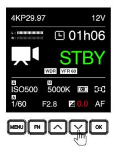
• **AF**: When focus is in **AF** mode (require to connect the autofocus lens), press **OK** to do auto focus.
