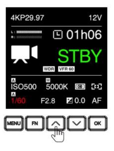
• **Aperture:** Press **F3** to set the aperture, then press **Up / Down** to adjust the value, and OK to confirm.
